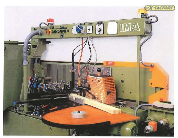
Hotmelt glue application unit 101.921 for veneer/plastic strip edging material and up to 8 mm wide lippings
